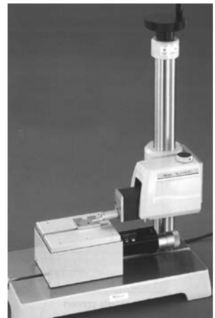
Measurement with a stand and leveling table
